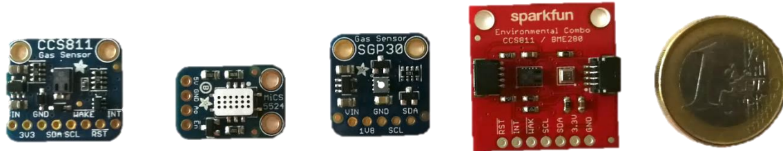
MOX-based IAQ sensor modules incl. breakout boards(from left to right): AMS CCS811, SGX MiCS-5524,Sensirion SGP30
