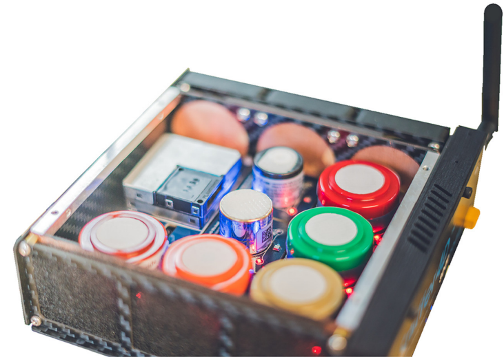
Sniffer 4D equipped with 5 Electrochemical sensors, 1 PID and 1 NDIR sensor.
