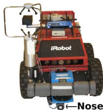
Continuous (open) sampling with a mobile robot
