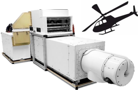
Helicopter-based Differential Absorption LIDAR (DIAL, Adlares GmbH)
